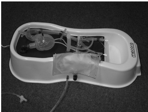
Figure 1. CoroSim ® , the pulsatile coronary artery model for pre- and post-evaluation of the participants.
